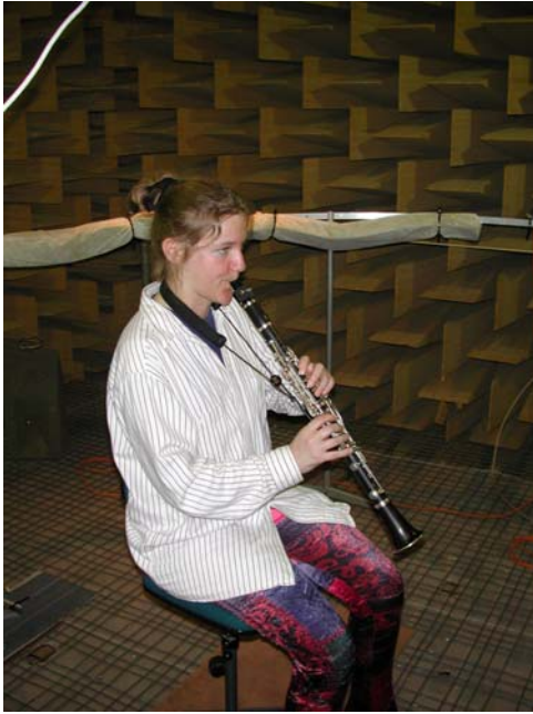
Fig. 1. Clarinet player during the directivity measurements in the anechoic chamber.
