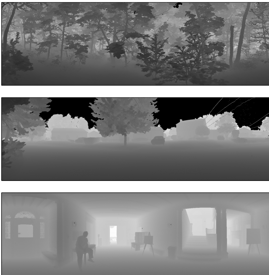
Figure 3.4: Samples from the Brown range image database by Huang and Lee. The gray values code for log-range values.
