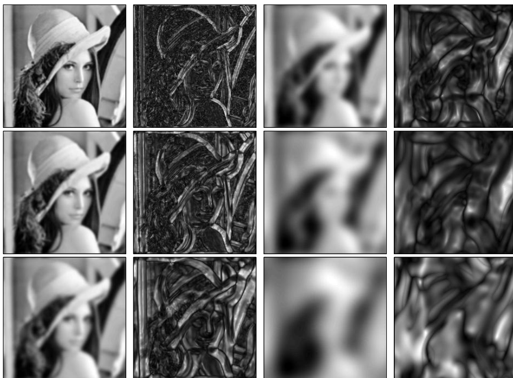
Figure 4.5: The first and third columns show scale-space images of “Lena” ( 226 \times 226 pixels) for exponentially increasing scales s \in [1; 16] . The second and fourth columns show the corresponding log-densities \log(\rho(\theta)) in jet space (a bright pixel corresponds to a high density). The densities \rho(\theta) are estimated at each pixel by computing the distance \theta to the manifold of blurred step edges and looking up the density values by \rho(\theta) = \theta^{-0.7} .
