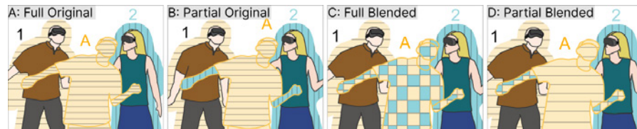
Figure 33: This figure illustrates how to control the motion of avatars through the Degree and Blending parameters. Subfigure A shows User 1 fully controlling Avatar A with their original movement (yellow). B shows User 1 (yellow) partially controlling Avatar A’s torso, while User 2 (blue) partially controls Avatar A’s arms, with original , unblended control. C shows User 1 (yellow) and User 2 (blue) fully blending the control over Avatar A. D shows a combination of control — User 1 (yellow) and User 2 (blue) partially blend control of Avatar A’s arms, while User 1 maintains full original control of Avatar A’s torso.
